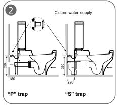
3 - Align the WC and secure it with the fixing nuts provided. We recommend tightening the nuts alternately to secure an equal fit against the wall
